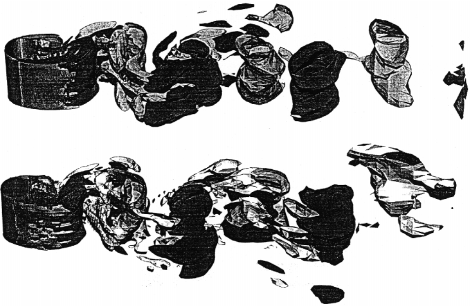
Figure 11. Axial vorticity distribution at Re = 20\,000 . Top: uniform flow; bottom: shear flow.
