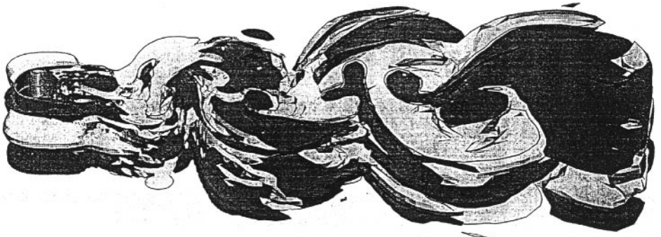
Figure 6. Streamwise vorticity distribution at Re = 10000 . Top: uniform flow; bottom: shear flow.
